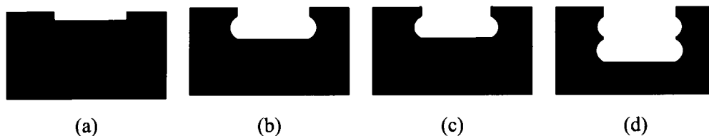
FIGURE 3. Etching and Deposition Steps of the DRIE Process. (a) Before Etching, (b) an Etching Step, (c) a Deposition Step, (d) Another Etching Step.
